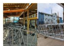
Angular towers for wind turbines Commenced March 2025; up to 140m for 3.15 MW turbines
