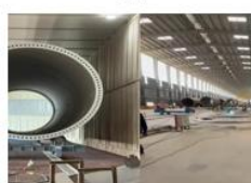
Tubular towers for wind turbines Commenced June 2025; sections up to 45m and 6m diameter
